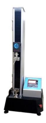
It is mainly used in various industries to perform material tensile strength testing, and is suitable for production workshops and laboratories.
