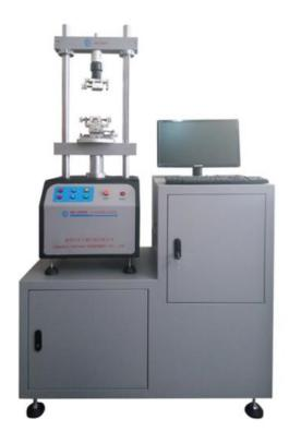
It mainly detects series of parameters such as insertion force, pull-out force, holding force and breaking force of various connectors, housings and terminals. Through data analysis by computer, it can accurately detect the load, stroke and corresponding curve, life curve, etc. of the connector., through the data report, summarize the test data. This provides a variety of scientific data for product quality testing. Widely used in automotive, wire, electronics, industry and other fields.
