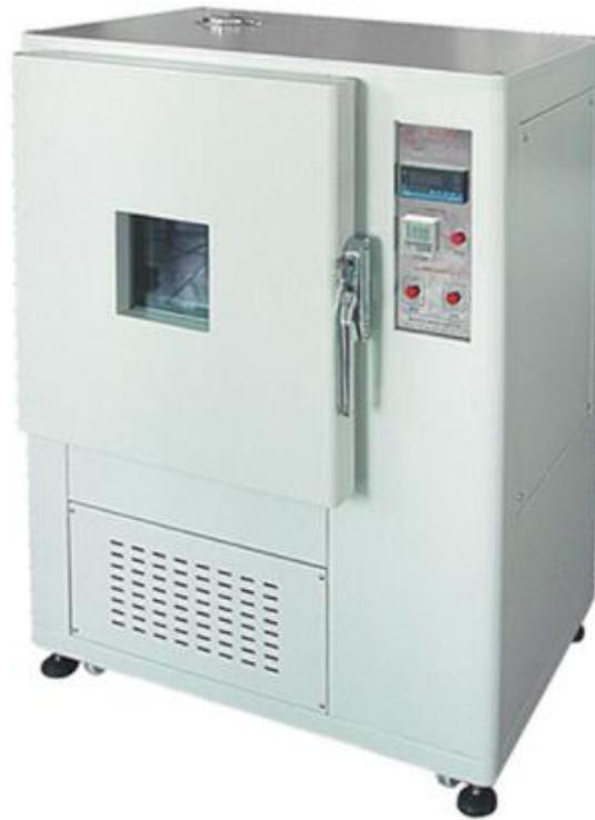
This instrument is mainly used for hot air aging test of rubber products, PVC wires and other products. It detects changes in aging extension and tensile strength of products and materials, and is suitable for quality control, laboratory and other places.
