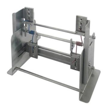
This instrument is mainly used to measure the performance of wire and cable under high temperature impact. It is suitable for round wire and cable, round insulated wire core, flat wire and cable insulation or sheath thermal shock test. It is the thermal shock performance of wire and cable industry. Test indispensable instruments.
