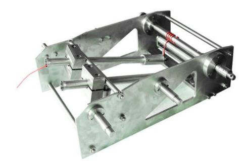
It is mainly used to test the dynamic bending performance of wire and cable under low temperature conditions. It is suitable for wire and cable or insulated core with outer diameter  $\leq 12.5$ mm, and flat wire and cable with short sleeve size less than 20mm or fan-shaped insulation that cannot be made into dumbbell. The core is an indispensable test device for the dynamic bending performance test of the wire and cable industry.
