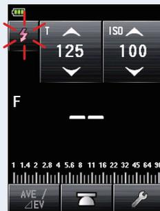
7. When the [Measuring Mode] Icon (
