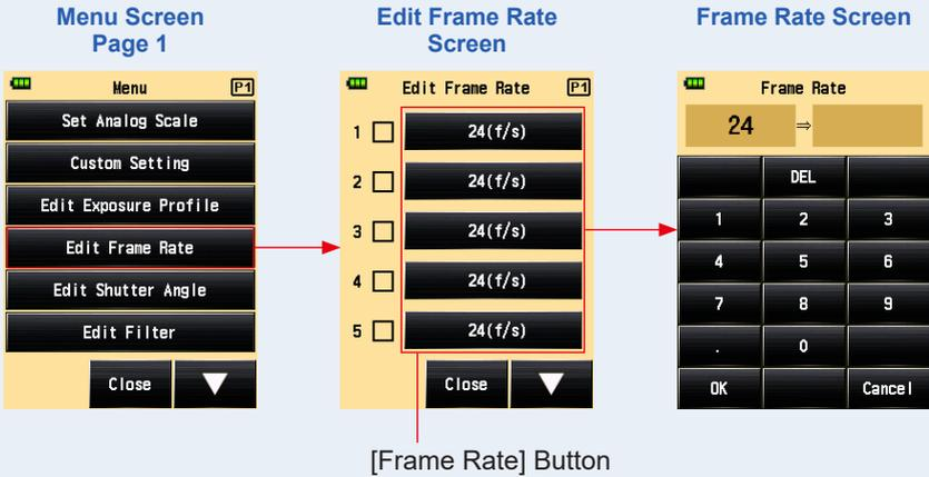
4. Input a numeric value in the Input Frame Rate Screen. (→ P11)
