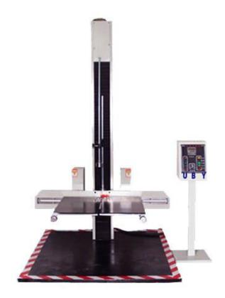
**Uses:** This device simulates the drop / fall of a finished product to evaluate damage. All the rhombohedrons, angles and faces of the package container can be tested.
