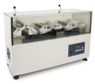
Footwear Sole Flexing Resistant Test Machine is used to measure the flexing resistance of shoe soles under continuous movement. Before test, plunge some holes at the maximum bending position, and mount specimen at both grips, one fixed, one movable. Specimen runs flexing owing to the movement of machine. After a certain test cycles, remove the specimen and check its difference of incision length.
