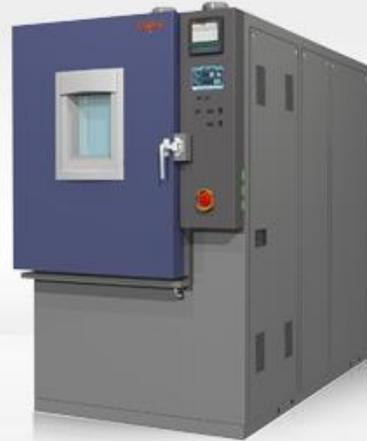
Today, the automotive industry accelerates electronic multi-functions. According to this trend, safety standards such as ISO26262 and IEC61508 require high environmental stress that is generated by thermal shock chambers for higher reliability of vehicle equipments.
