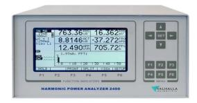
High-performance precision in both single and three-phases: a wattmeter, oscilloscope, and power spectrum analyzer in one. The 2400 power analyzer measures, computes and displays critical power variables so you can concentrate on more efficient & reliable testing. The 2400 Series provides simultaneous, precise voltage and current measurements while monitoring and displaying the power parameters you need in the format that best fits your application.
