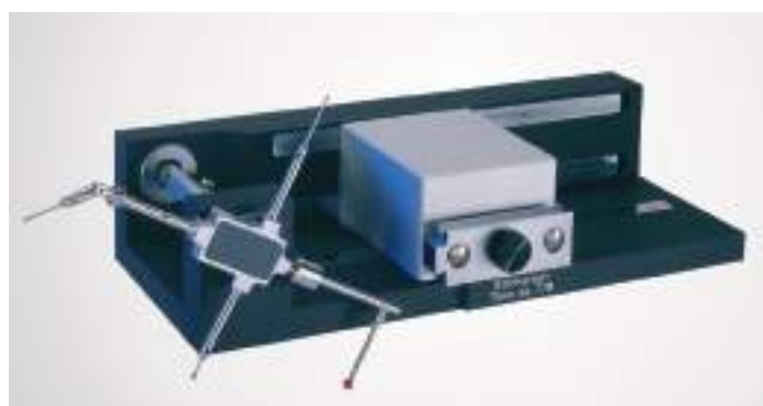
Device for balancing probe arms
