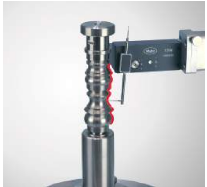
3D contour standard KN100S
