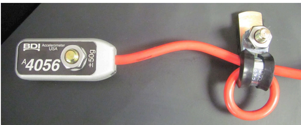
Figure 11: Sensor mounted with cable strain relief loop
