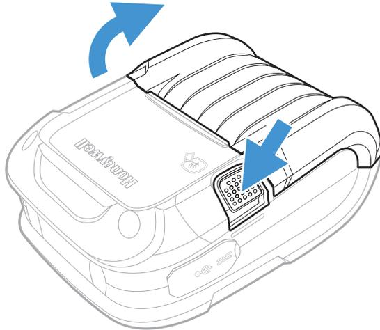
2. Open the external media door located under the supply hubs.
