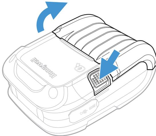
2. Slide and hold open the supply hubs.
