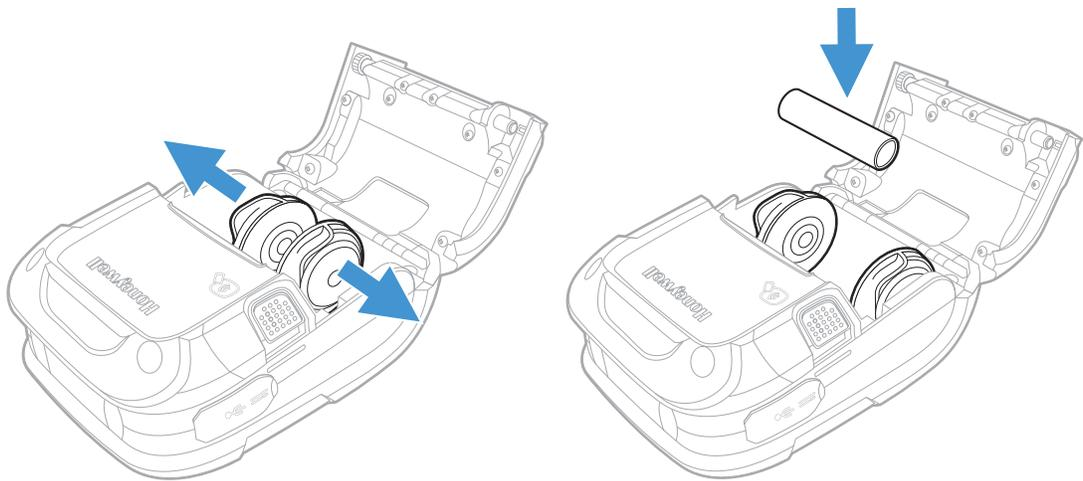
4. Insert the media through the external media door and through the printer.
