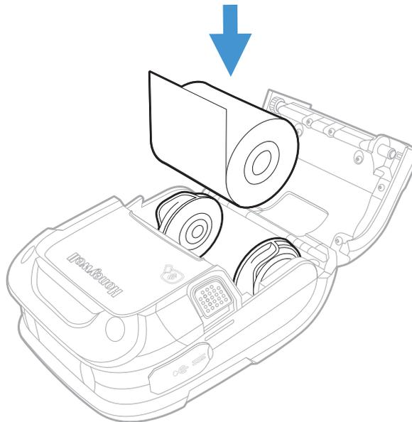
4. Allow the supply hubs to retract onto the paper roll and press the cover down until it latches.
