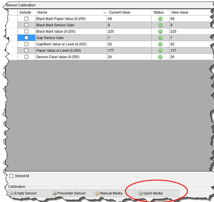
5. The printer feeds media while the sensor is calibrated. If the calibration is not successful, repeat the procedure or use [Manual Media Calibration](#).
