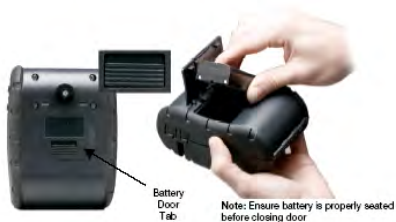
FIGURE 2: INSTALLING THE BATTERY CARTRIDGE
