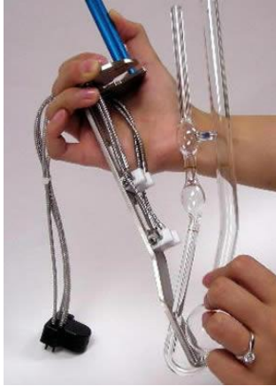
Figure 6. Inserting Base of Viscometer
