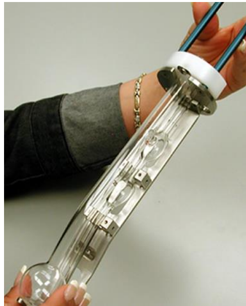
Figure 9. Viscometer Tube Completely Inserted in the Optical Sensor Assembly with Teflon ® Ring. (Optical wires are not shown for illustrative purposes only.)
