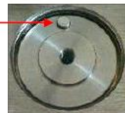
Sample Tray Drive & Index Pin
