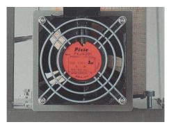
Use an external fan for faster response and more accurate measurement. It is in combination with this fan that the maximum capability of measurement for temperature and humidity can be achieved.
