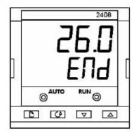
② To reinitialize the program, press and hold the key for 2 seconds (the RUN LED goes out). The regulator is then ready to restart a test.
