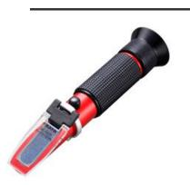
Brix 0.0 to 18.0% Good for measuing fresh fruit juice, water-soluble cutting fluid and etc.
