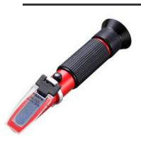
Brix 45.0 to 82.0% Good for measuring objects with medium-high concentration such as jam, cooking oil, marmalade and etc.
