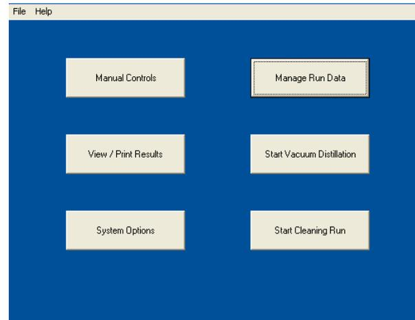
**Manual Controls:** This area is used for manually operating some aspects of the equipment. Vacuum level, vapor and pot temperatures can be monitored. This is useful for checking the equipment function and performing maintenance.
