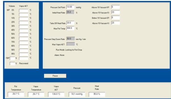
On the left side of the screen is a display of the results for this distillation including IBP (Initial Boiling Point), various distillation points and the FBP (Final Boiling Point).
