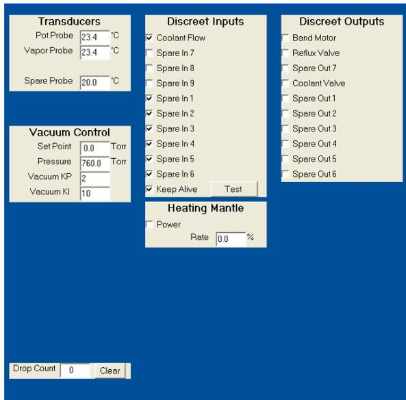
**Transducers** show the current temperatures for the pot temperature probe and the vapor temperature probe.
