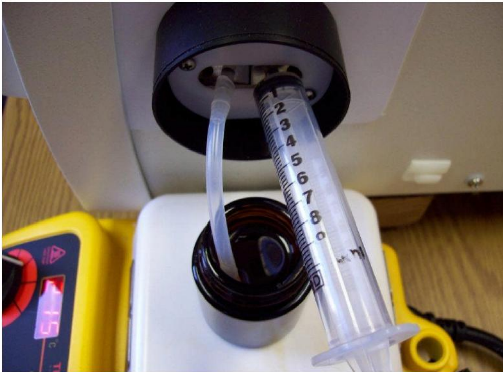
Figure 7.12 Sample is Hot. Notice the syringe; it is to be used to pull the sample into the density meter rather than being pushed
