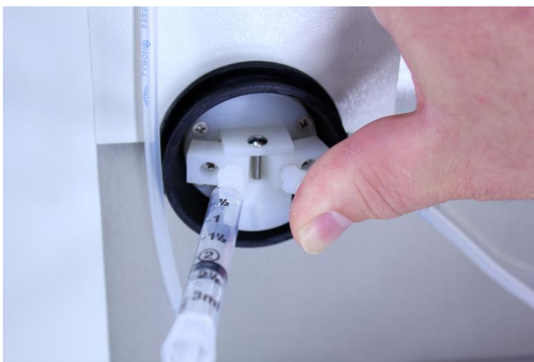
Figure 5.4 Checking the Filling Nozzles for Air Tightness
