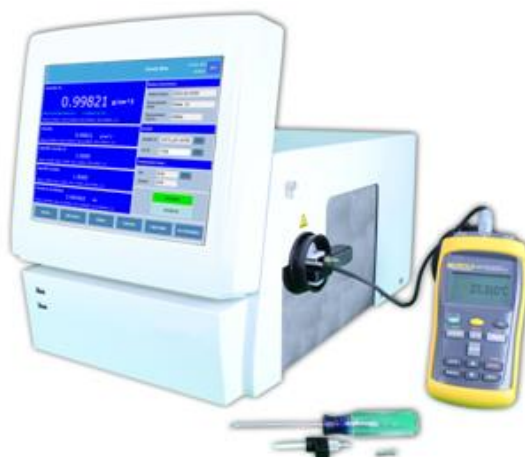
Figure 9.10 Temperature verification with a certified Fluke Hart Thermometer
