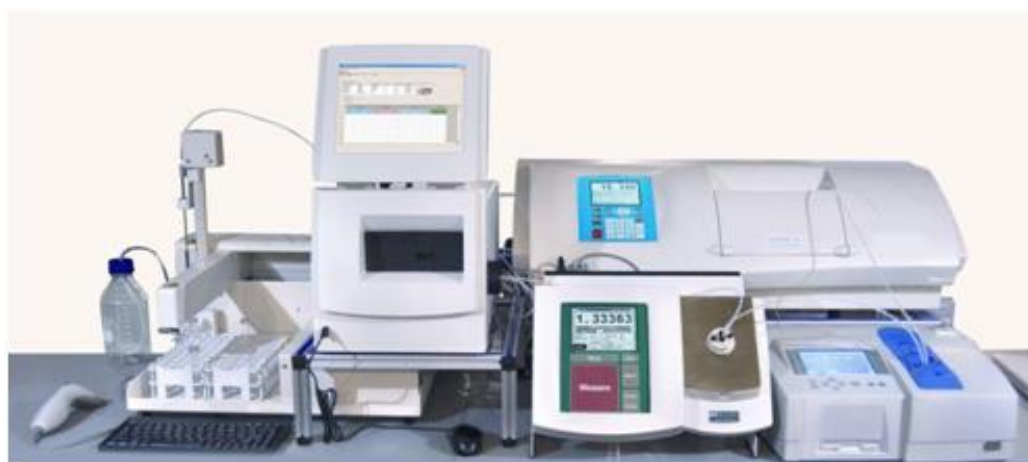
Fig.12.15 A Flavor-Fragrance System for the Simultaneous Measurements of Specific Gravity, Refractive Index, Color, and Optical Rotation. As shown this system can handle up to 120 samples.
