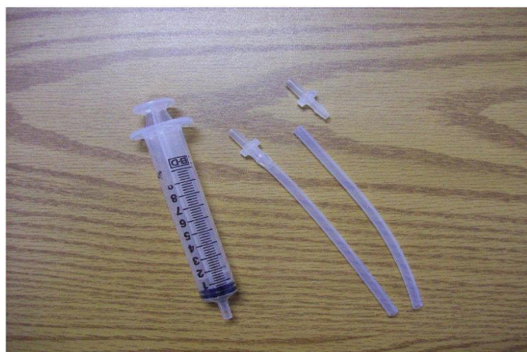
Figure 7.11 Items to be used for viscous and solid samples (For the new system, the two plastic hose barbed male Luer adaptors are not used)
