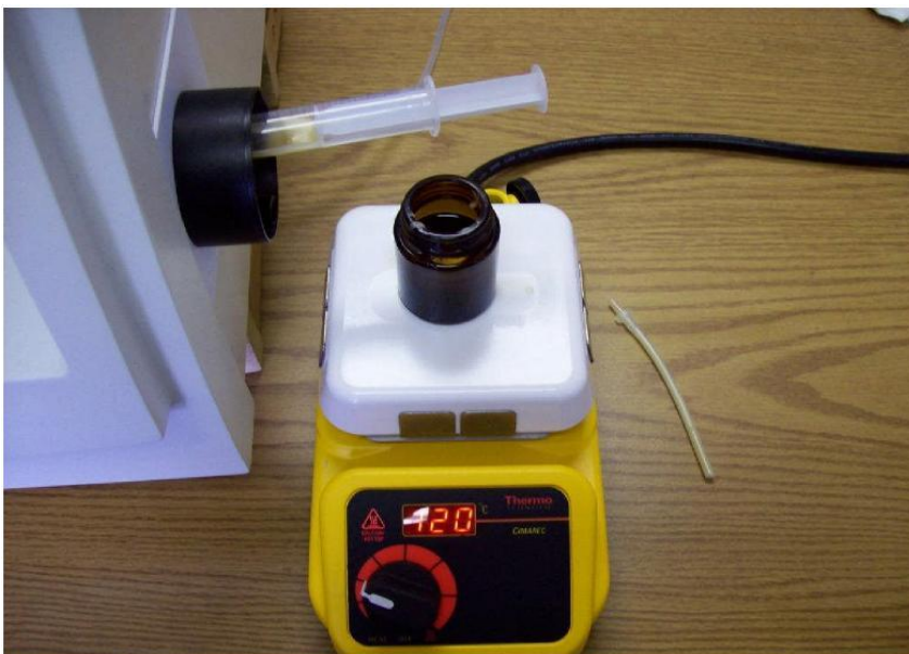
Figure 7.14 Here the syringe's plunger has been drawn back and the molten sample pulled up into the tubing and into the U-tube. The molten sample will harden inside the cheap tubing which is thrown away.
