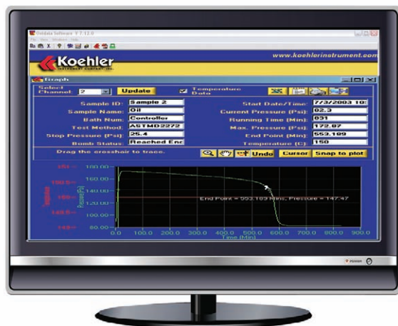
Oxidata® software automatically detects the break point and induction period.
