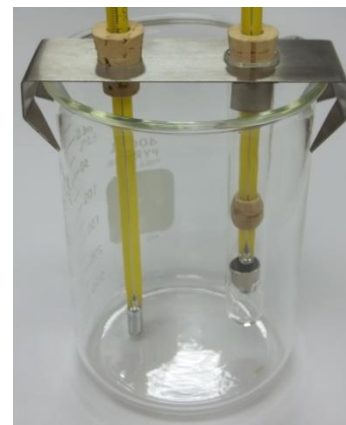
Figure 5: Beaker and Test Tube Apparatus Assembly
