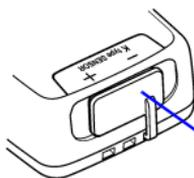
Insert the protective cap into the sensor connectors when not in use.
