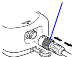
To remove the RS-232C cable, grip the connector coupling and pull it straight out to remove it.
