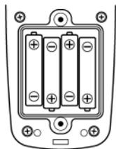
1. Remove back cover screw to remove cover. Verify polarity and install four new LR03 alkaline batteries.
