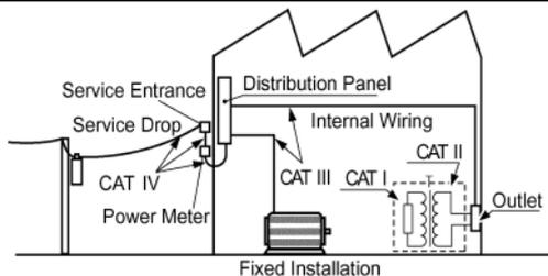
Higher-numbered categories correspond to electrical environments with greater momentary energy, so a measurement product designed for CAT III environments can endure greater momentary energy than one designed for CAT II. Using a measurement product in an environment designated with a higher-numbered category than that for which the product is rated could result in a severe accident, and must be carefully avoided.
