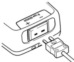
Aligned polarity of both connectors to insert the sensor connector.
