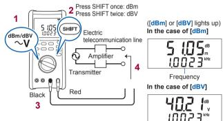
Example: Measuring the [dBm] cable loss
