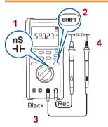
The open terminal voltage is approx. 2.5 V or less. The measurement current (DC) is approx. 96 nA. (p. 87) To avoid damage to the measurement object, check the specifications before use.
