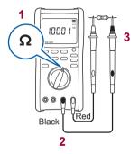
Measurement of inductors, including motors and transformers, may cause unstable auto-range switching. In such a case, set the range manually (p.55). Moreover, if a capacitive component is connected across the object under measurement, its measured value may be incorrect.
