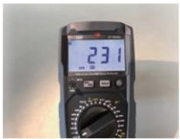
hFE triode measurement function
