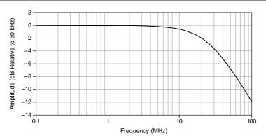
Figure 2. NI 5751 Characteristic Frequency Response
