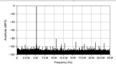
Figure 4. NI 5751 Characteristic Noise Density, Spectrum-64 k Samples
