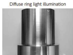
Difficult to detect scratches due to glossy metal surface
