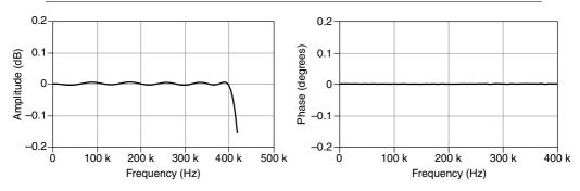
Figure 4. 10 MS/s Frequency Response, Measured
