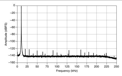
Figure 6. PCI-5922 Dynamic Performance with 10 kHz Input Signal, Measured, 1 MΩ, 2 V<sub>pk-pk</sub> Range, 100 kS/s, Unbalanced Differential, 10,000-Point FFT with 10 Averages
