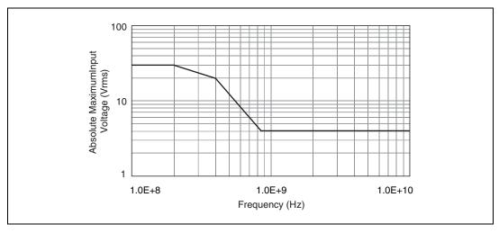
Figure 5. NI 5191 Derating Curve
