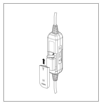
Figure 1. Installing the 9 V Battery in the NI 5191
