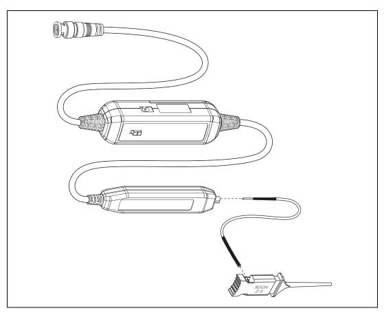
Figure 4. Connecting a Pincer Clip to the NI 5191
