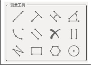
Point spacing,point line spacing,line spacing,center distance,arc, circle,Angle,rectangle,polygon measurement, calibration function,automatic edge searching
