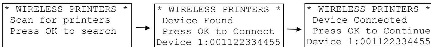
When you have connected successfully the printer's green status light will turn on. Pressing the **PRINT** key will now display the PRINT MENU.
