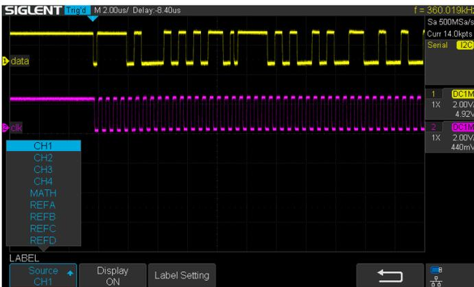
When multi-channel measurement is used, corresponding labels are set for different sources to facilitate observation and reading.
