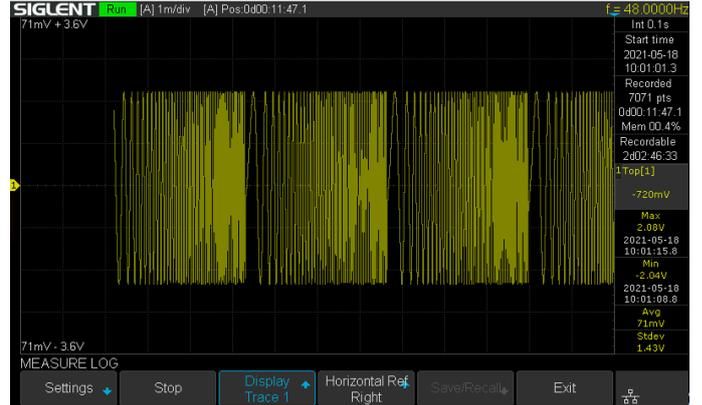
The measurement Logger is designed to collect measurement values for a long time. The data is logged in memory. After logging is complete, the data can be saved into the internal flash or external U disk.
