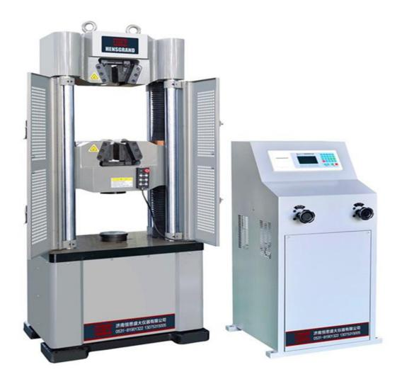
WE-100D Digital Display Hydraulic Universal Testing Machine
