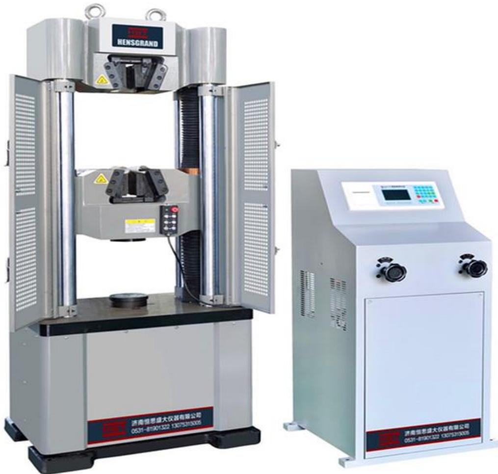
WE-200D/WE-300D Digital Display Hydraulic Universal Testing Machine
