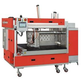
The new **TP-702CTRS** is designed to strap specialty boxes, including crash lock boxes, four corner tray, and other folded type boxes from shingled-stream folder gluer output. The clever side-pusher and backstop designs ensure of the best stack condition after strapping and protect delicate boxes from damage without sacrificing its high speed. TP-702CTRS is an efficient squaring and strapping solution for specialty folder gluer products.
