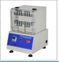
A rectangular strip of coated fabric is folded twice so that its long edges meet forming a strip measuring 125mm\*12.5mm. This folded strip is mounted between a pair of flat grips, one of which reciprocates, causing the folded test piece to be sent outwards five times per second. This high-speed folding of the test piece is continued for either a pre-set number of cycles or until damage to the test piece is apparent.
