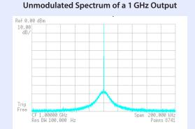
The SG380 Series outputs exhibit low phase noise and low spurious content. In this direct measurement taken with 100 Hz RBW, the noise floor of the spectrum analyzer dominates over most of the 200 kHz span.
