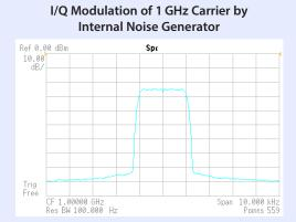
Option 03 allows I/Q modulation of carriers from 400 MHz to the upper frequency limit of your instrument. Two signal sources may be used for I/Qmodulation: external I & Q inputs or an internal noise generator. The external I & Q BNC inputs are on the rear panel. The internal noise generator has adjustable noise bandwidth. Shown here is a 1 GHz carrier being modulated by the internal noise generator with 1 kHz noise bandwidth.
