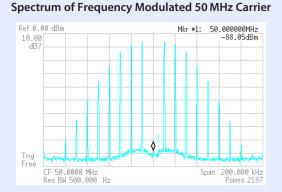
Outputs below 62.5 MHz are generated by directdigital synthesis with a sample frequency of 1 GHz. In this example, a 50 MHz carrier is frequency modulated at a rate of 10 kHz and a deviation of 24.0477 kHz, for a modulation index  $\beta = 2.40477$ . The carrier amplitude is proportional to the Bessel function  $J_0(\beta)$ , which has its first zero at 2.40477.
