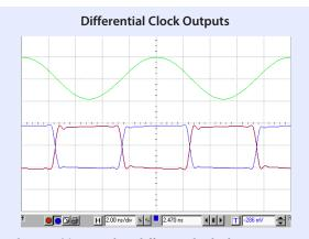
Option 01 provides differential clock outputs in addition to sine outputs. The clocks have transition times of about 35 ps. Both the offset and amplitude of the clock outputs can be adjusted for compliance with standard logic levels. Shown here at 2 ns/division: 100 MHz front-panel sine wave output (top trace) and differential clock outputs (bottom traces). The displayed transition times are limited by the 1.5 GHz bandwidth of the oscilloscope.
