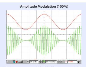
The frequency range of the SG380 Series extends from DC to 2 GHz, 4 GHz or 6 GHz (depending on model). All of the analog modulation modes also extend to DC allowing your SG380 to perform function generator tasks. Shown here is a 20 kHz carrier being amplitude modulated by a 1 kHz sine.
