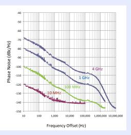
The SG380 Series always synthesizes a frequency in the top octave and digitally divides to generate outputs at lower frequencies. Doing so creates phase noise characteristics which scale with output frequency by 6 dB/octave or 20 dB/decade.
