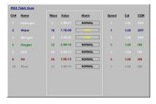
**Table mode** provides a readout of mass, scaling factor, and true partial pressure. The display shows the peak heights and alarm status of up to 10 masses. The electron multiplier can be independently set on or off for each mass. This allows the user to view minor species even in the presence of high total pressure.
