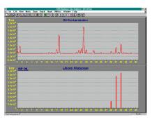
Library mode contains a comprehensive list of gases that can be used to compare against the current spectrum. A search mode allows you to select up to 12 masses and identify and display (numerically and graphically) the intensity of all gases that contain these masses.
