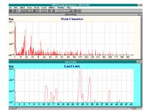
**Multi-head operation** is available when more than one RGA is needed for analysis. Up to eight heads can be monitored simultaneously from the software.
