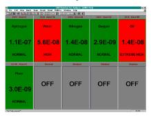
**Annunciator mode** is provided for conveniently monitoring up to 10 masses. If a particular mass has tripped its preset alarm, the large box will turn red indicating a problem. An audible alarm will also be present until the mass falls back within its preset limits. This mode is most often used for Go/No-Go testing.
