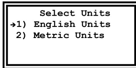
With English units selected, the lift and drag forces are displayed in pounds (lb) and the wind speed in miles per hour (MPH). Selecting metric units displays the lift and drag forces in kilograms (kg) and the wind speed in kilometers per hour (KPH). Since L/D is unit-less the units are not displayed. When the controller is powered up the display units default to English.
