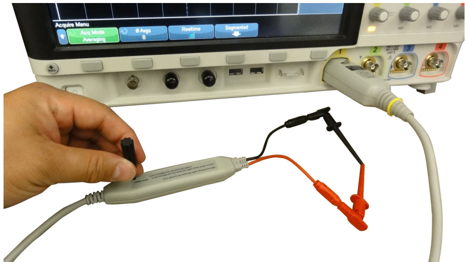
Figure 7 Adjusting the Offset Using the Supplied Tool
