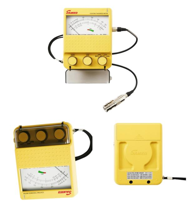
One pole type probe for coating and lining on the-spot-site use
