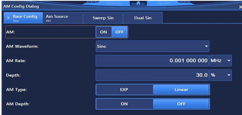
Fig.2.32 Amplitude Modulation Configuration Dialog
