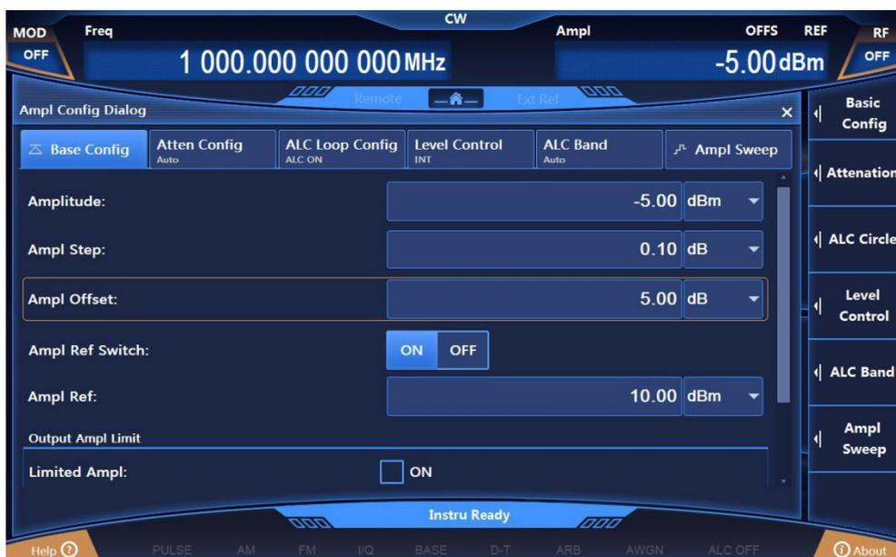
Fig.2.21 Ampl Offset of 5dB
