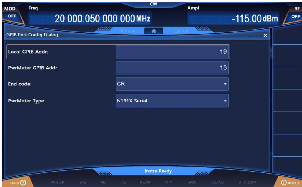
Fig.2.9 GPIB Port Setting
