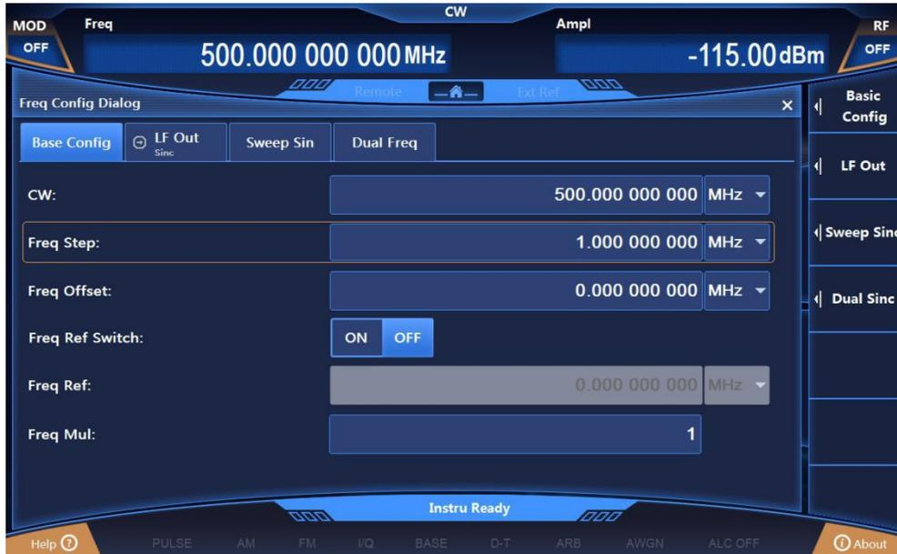
Fig.2.16 Setting CW to 500MHz at a Step of 1MHz
