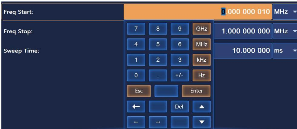
**Method 2:** Turn the front panel knob, when the 'Freq Start' data input box is selected, press the knob to make the box 'Editable', then enter data and edit it. After editing, press the knob again to make the data input box selected, and then operate other controls by turning the knob.
