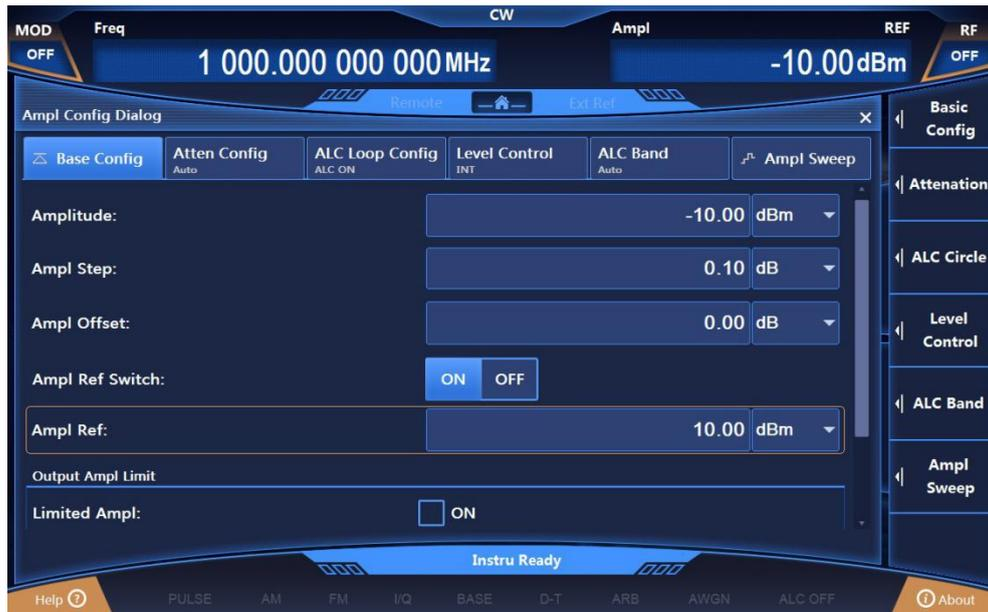
Fig.2.20 Power Level of 0dBm with Reference of 10dBm
