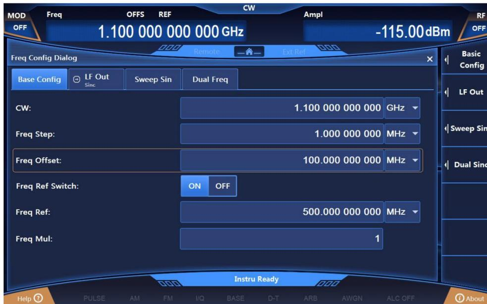
Fig.2.18 Setting Freq Offset to 100MHz
