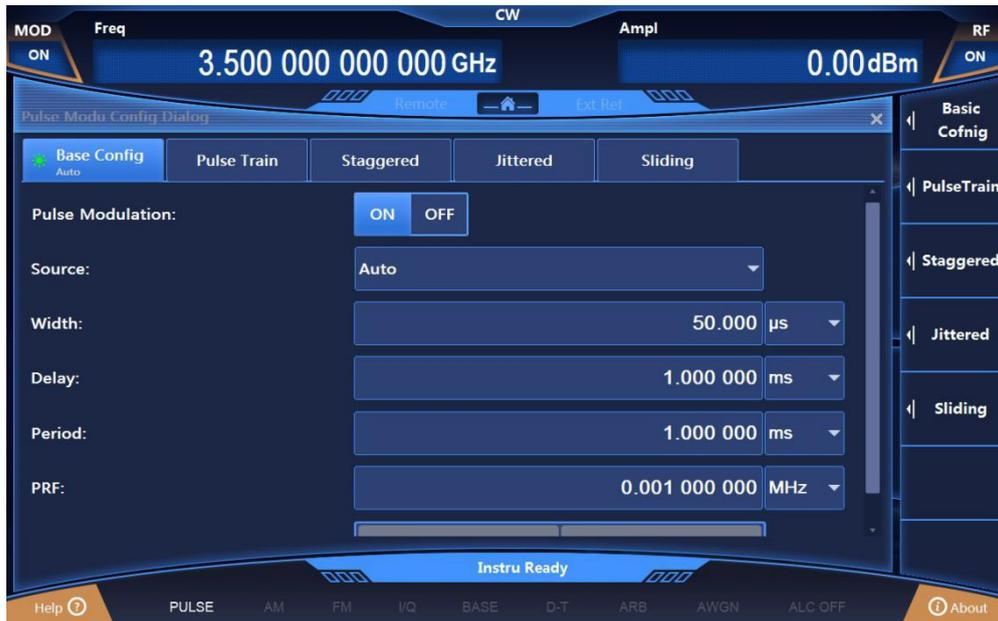
Fig.2.23 Setting of Pulse-modulated Signals
