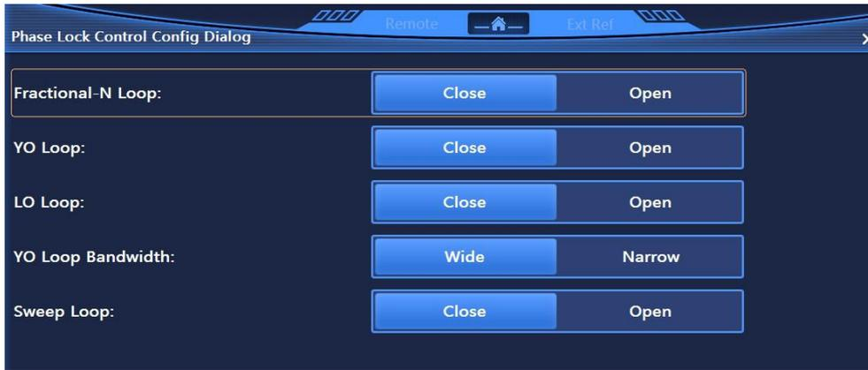
Fig.4.57 Phase Locking Control Dialog
