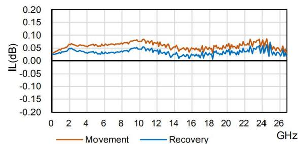
*\*Under condition: Data tested from 3.5mm ECAVNA test cable, at bent 360° with 10cm diameter.*
