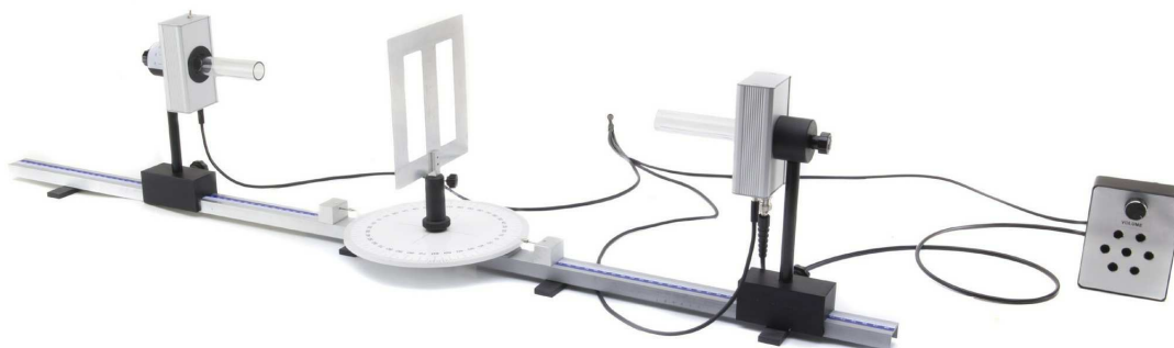
Fig. 1: Set-up for the diffraction experiment (double-slit).
