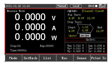
Figure 5-2 <QC3.0> Setting and Display Interface
