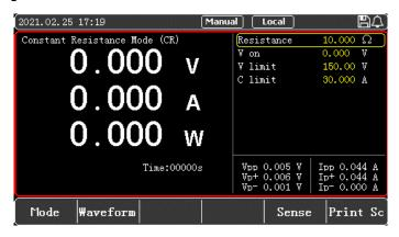
Figure 4-1-3-1 Setting Interface of CR Mode
