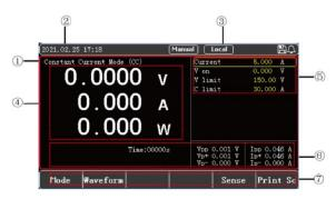
Figure 3-2 Interface of Measurement
