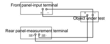
Figure 7-3 Wiring Diagram of Remote Compensation
