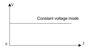
Figure 4-1-2-2 Relationship of Voltage and Current in CV Mode
