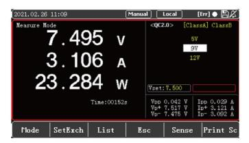
Figure 5-1-2 QC2.0 Measurement Interface in CV mode
