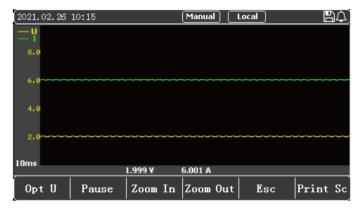
Figure 4-4 Current and Voltage Waveform Display in CV Mode
