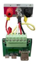
Figure 1-2-3 Connection of Terminal and Quick Charge Test Board (UTL8511C)
