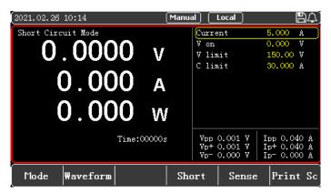
Figure 4-2-9-1 Interface of Short-Circuit Mode
