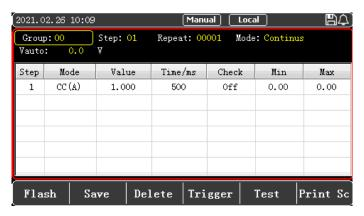
Figure 4-2-2 Setting Interface of List Mode
