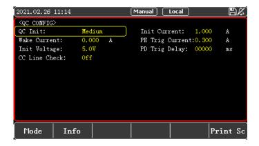
Figure 5-7 < Quick charge Setting> Interface
