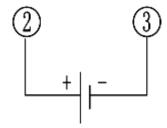
3. Wiring method for test result output (need external power supply)
