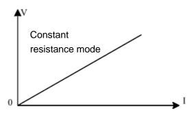
Figure 4-1-3-2 Relationship of Voltage and Current in CR Mode
