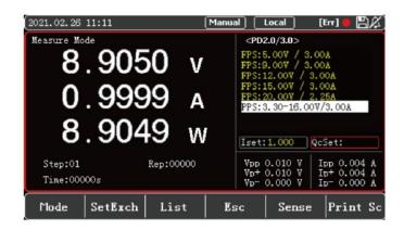
Figure 5-4-2 <PD2.0/3.0> Setting and Display Interface
