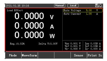
Figure 4-2-7-1 Interface of Load Effect Mode
