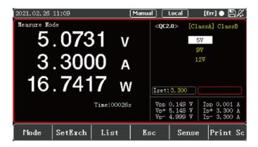
Figure 5-1-1 <QC2.0> Setting and Display Interface
