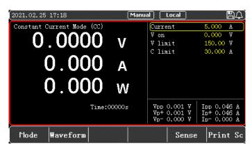
Figure 4-1-1-1 Setting Interface of CC Mode
